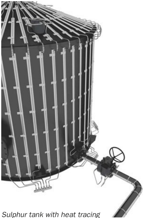
Sulphur tank with heat tracing
