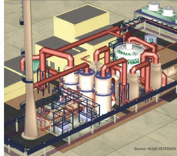
Fig. 5: Crimea Titan 1,800 t/d sulphur-burning sulphuric acid plant with >97% heat recovery
