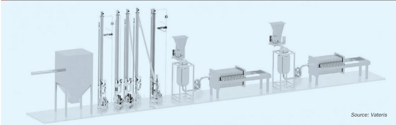
Fig. 1: Schematic of Vateris’ pilot process. This novel patented technology combines gypsum, potassium hydroxide and captured industrial carbon dioxide to produce two valuable products: high-purity SOP fertilizer and a specialist calcium carbonate material for the construction sector.
