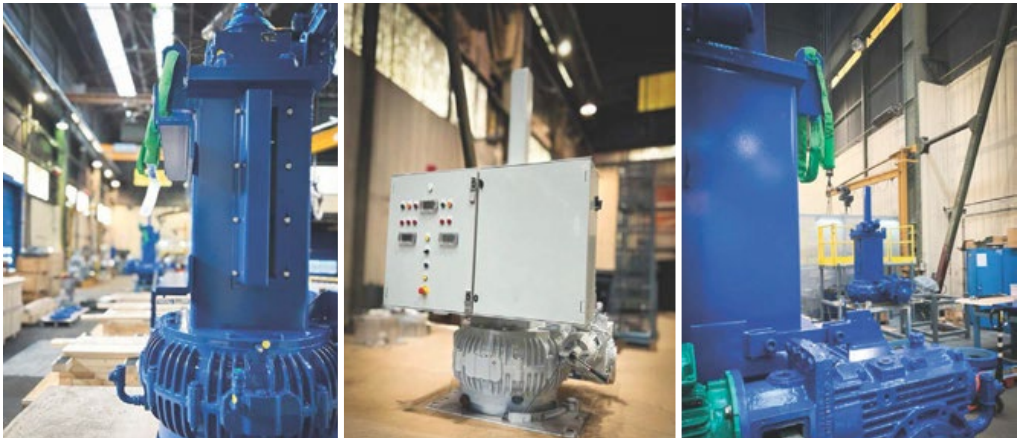
CMD Gears drive heads: purely mechanical model (blue paintwork) for a French OEM who will then integrate the electrical components; complete model (white paintwork) equipped with a control cabinet, motors and sensors for direct delivery to the customer.
