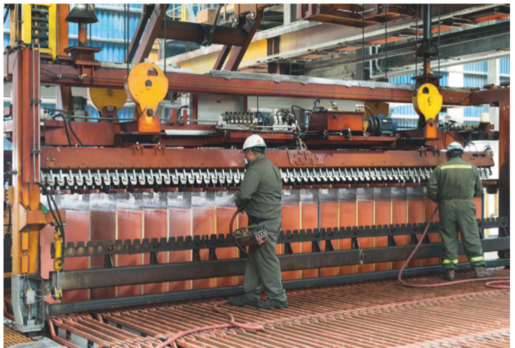
Copper cathodes at an SX/EW plant, Antofagasta, Chile
