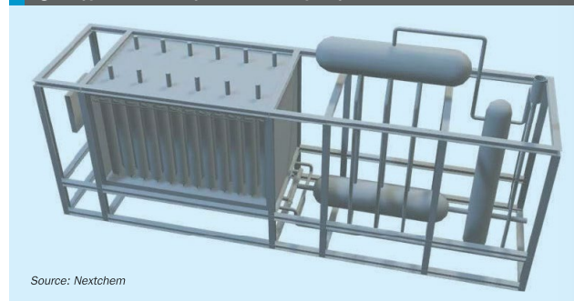
Fig. 1: Typical modular layout for small capacity NX eBlue™ reactor
