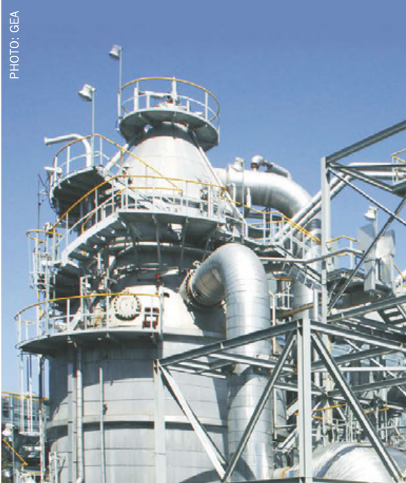
Operational GEA crystalliser at a fertilizer production plant.
