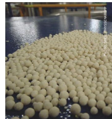
Fluidised-bed granulated Urea-ES® fertilizer (43-0-0-7S), Leuna, Germany.
