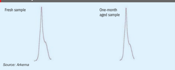
Fig. 3: CustoFloat M (experimental version): analysis spectra showing more stability after one month
