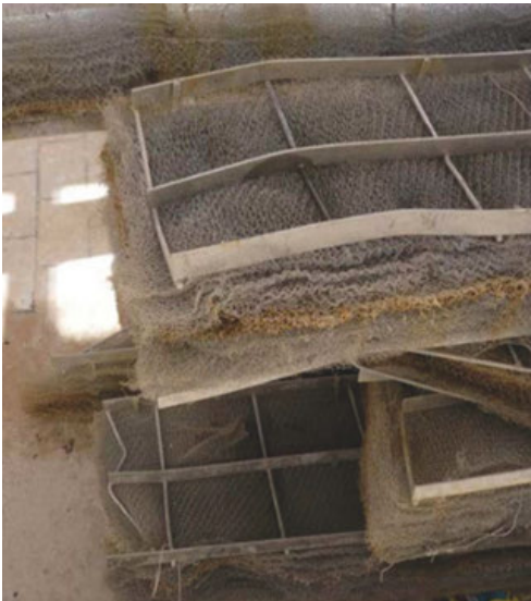
Photo 10: Demister sections damaged a lot.
