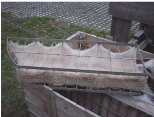
Photo 3: Shrunken ETFE mesh section.
