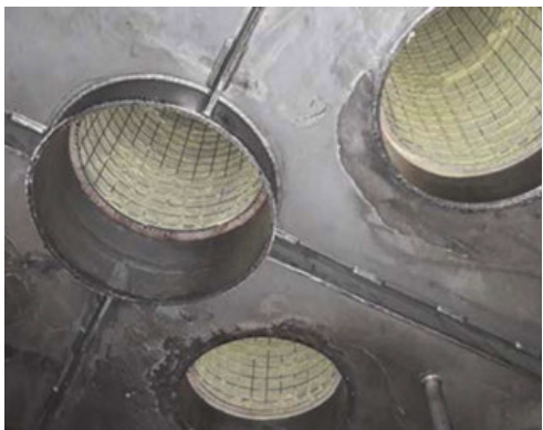
Photo 5: Sulphur sublimation in a standing filter.
