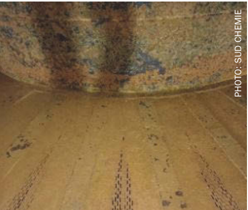
Active pyrosulphate melt migration and deposition on bottom gratings/grids, blocking the gas path.
