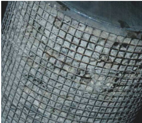
Photo 8: Glass fibre corrosion by HF at top of filter.
