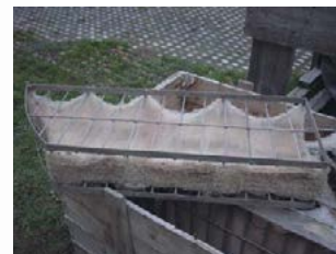
Photo 3: Shrunkn ETFE mesh section.
