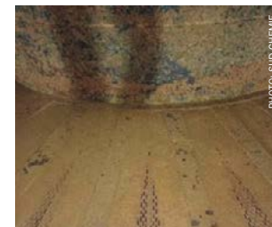
Active pyrosulphate melt migration and deposition on bottom gratings/grids, blocking the gas path.
