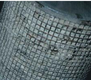
Photo 8: Glass fibre corrosion by HF at top of filter.
