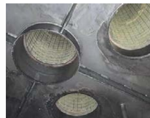
Photo 5: Sulphur sublimation in a standing filter.
