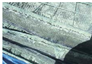
Photo 1: Sulphated demister sections.
