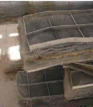
Photo 10: Demister sections damaged a lot.
