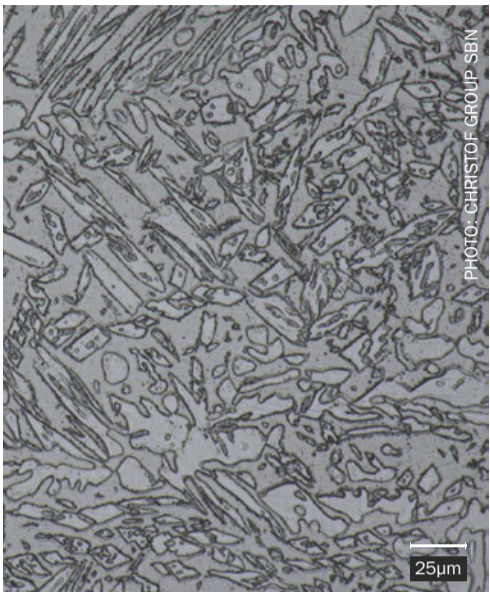
Fig. 1: Optical microscopy image of microstructure of UNS S32906 sample produced by WAAM, after heat treatment. A balanced dual-phase composition, with near-equal proportions of ferrite and austenite phases distributed consistently across the deposited bulk is presented. Magnification 1000x.
