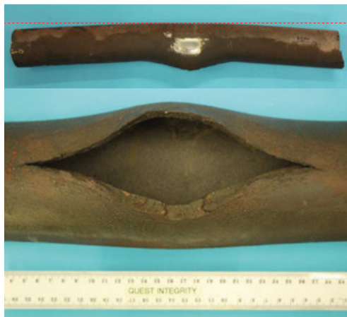
Fig. 2: Example of a creep rupture in a superheated steam tube (material: 9Cr1MoV). Note the “fish mouth” rupture and deformation. The polished patch indicates a location of metallurgical replication.
