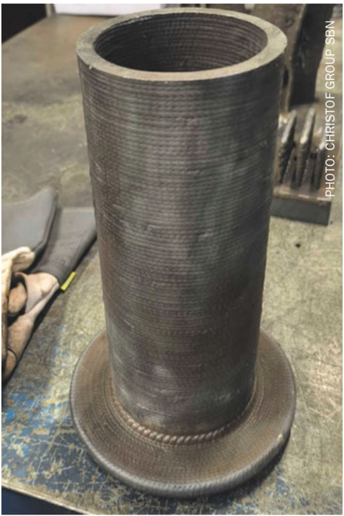
Fig. 2: A flange made with WAAM technology. UNS S32906 filament, with diameter of Ø1.2 mm
