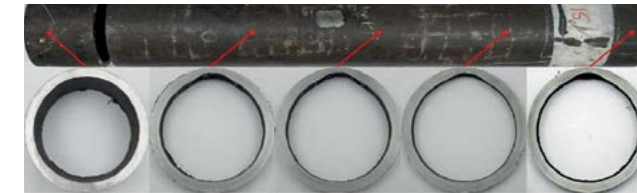
Fig. 3: Example of a localised metal loss observed in a convection section tube (material: carbon steel). The polished patch likely indicates a location of metallurgical replication.
