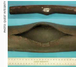
Fig. 2: Example of a creep rupture in a superheated steam tube (material: 9Cr1MoV). Note the "fish mouth" rupture and deformation. The polished patch indicates a location of metallurgical replication.
