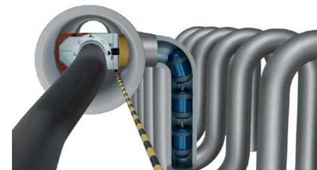
Fig. 4: Conceptual image of an FTIS® intelligent pig entering a coil connected to a manifold by way of the header delivery system (HDS) developed by Quest Integrity.
