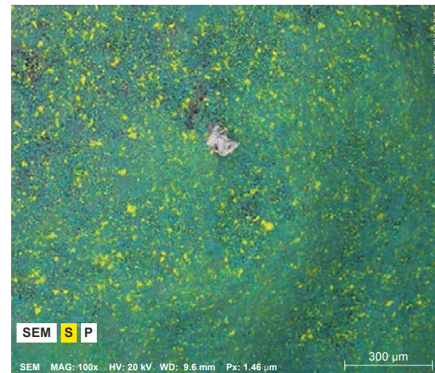
Fig.1 Scanning electron micrograph (energy dispersive x-ray) imaging of the interior of a Phosphate+MST® granule showing MST® (yellow) distributed throughout the phosphate (blue).
