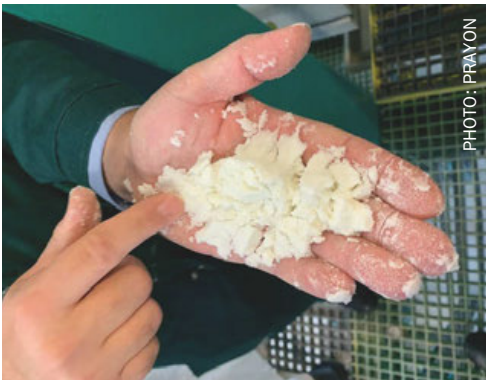
Di-calcium phosphate (DCP) filtration cake generated by Prayon’s new fluorosilicic acid (FSA) valorisation process.
