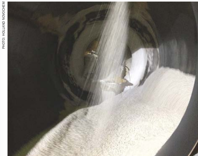
Drum coating of fertilizer granules.
