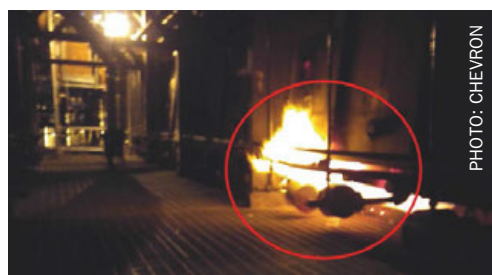
Fig. 1: Fire escaping the furnace box
