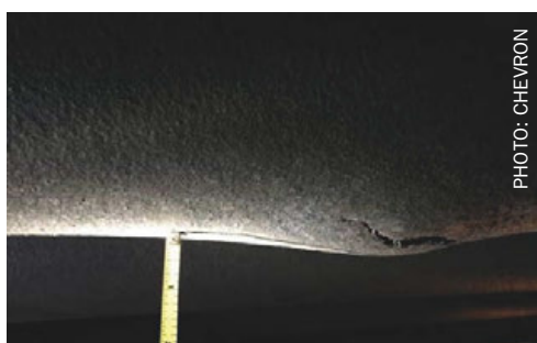
Fig. 4: Photograph of tube crack and bulging
