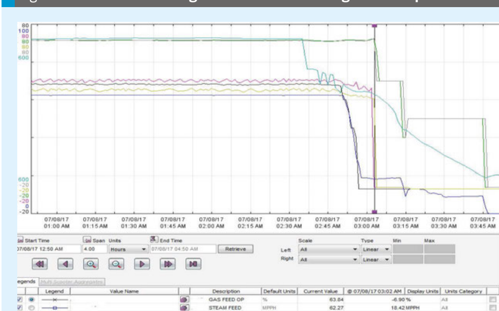
Fig. 3: Process trend showing steam flow and natural gas FCV output
