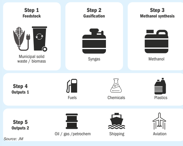
Fig. 1: Biomass / waste route to sustainable methanol production
