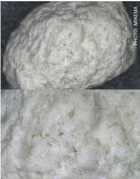
Main image: The creation of fertilizer dust during handling, transit and storage poses serious health risks and degrades the product. This can be prevented using coatings that preserve the integrity of fertilizer granules. Above: Microscope image of a fertilizer granule at 50x (top) and 100x (bottom) magnification. Tiny particles and crystals on the surface can potentially turn into fine dust.
