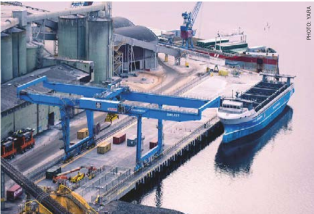
Yara Birkeland is the world's first fully electric and autonomous container vessel.
