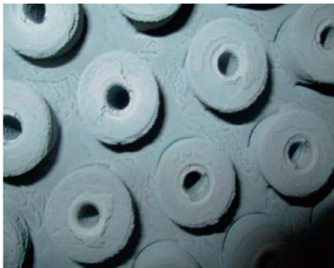
Blocked orifice plugs in circulation heater bottom and top liquid divider blockage.
