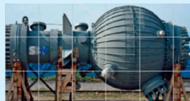
The HP scrubber reduces the ammonia content in the inert stream.
