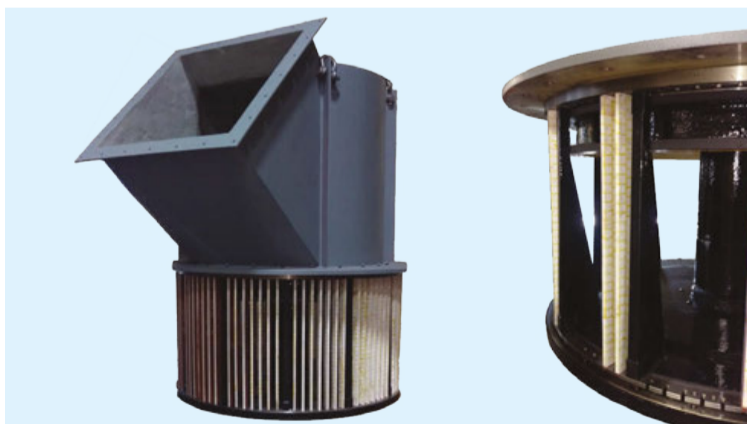
Reinforced classifier with wear protected VBC rotor (main photo, left). The use of ALOX tiles and polyurethane coatings (close up, right) prevents abrasion in direct impact areas.
