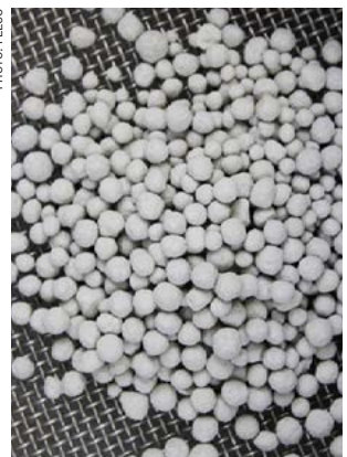
PHOTO: FIECO Finished monoammonium phosphate (MAP) fertilizer.
