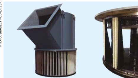
PHOTO: BRADLEY PULVERISER Reinforced classifier with wear protected VBC rotor (main photo, left). The use of ALOX tiles and polyurethane coatings (close up, right) prevents abrasion in direct impact areas.
