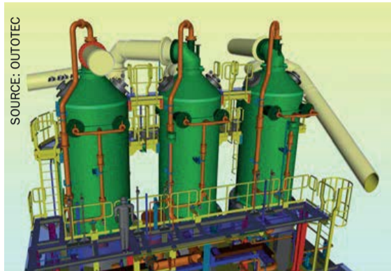
Fig. 12: Drying tower and absorption tower modules.
