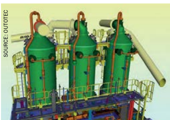
Fig. 12: Drying tower and absorption tower modules.
