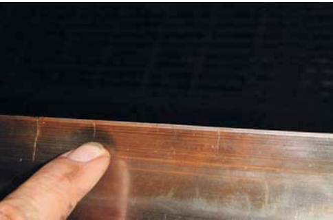
Fig. 5: Edge cracks developing.
