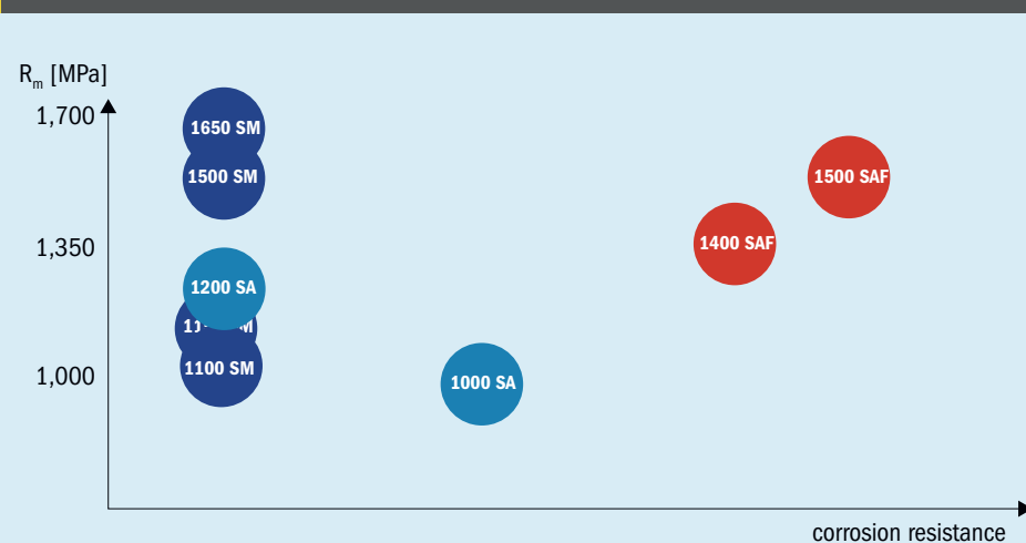
Fig. 10: Steel belt grades tensile strength versus corrosion resistance
