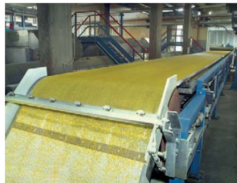
Fig. 8: A steel belt cooler producing sulphur pastilles.
