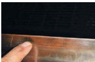
Fig. 5: Edge cracks developing.
