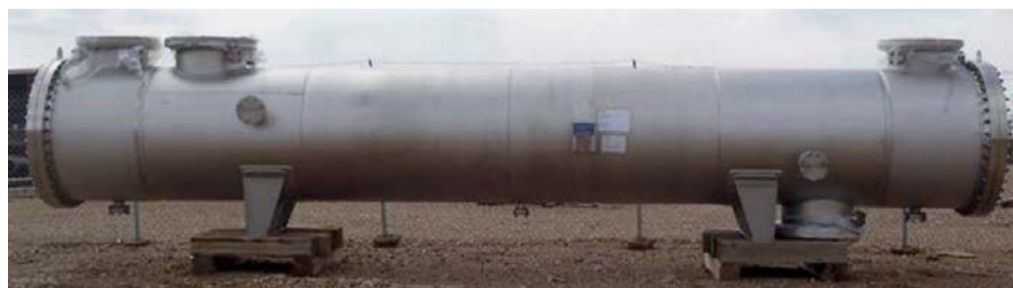
Acid cooler fabricated in NORAM SX™ alloy.
