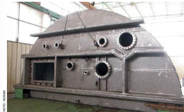
Assembly of a pump tank (half) fabricated in NORAM SX™ alloy.
