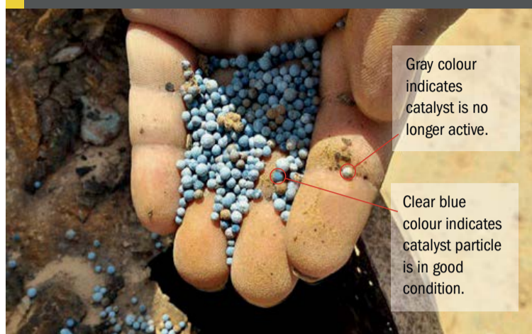
Fig. 8: Contaminated vs non-contaminated catalyst
