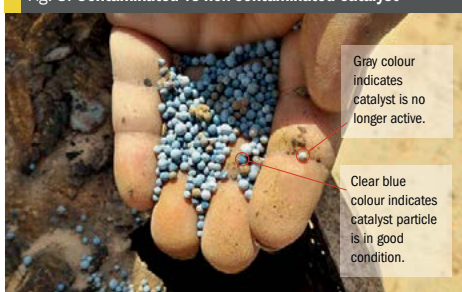
Fig. 8: Contaminated vs non-contaminated catalyst
