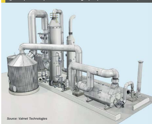
Fig. 3: Sulphuric acid plant model at Metsä group Bioproduct mill, Äänekoski, Finland
