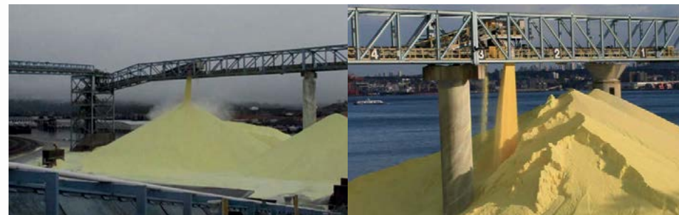
Figure 1: Sulphur stacking operation from conveyor tripper stacking operation at 4,000 t/h without IPAC dust suppressant (left) and with IPAC dust suppressant (right). Of particular note in the picture on the left is that it is a wet, rainy day, indicating the poor ability of water to suppress dust.
