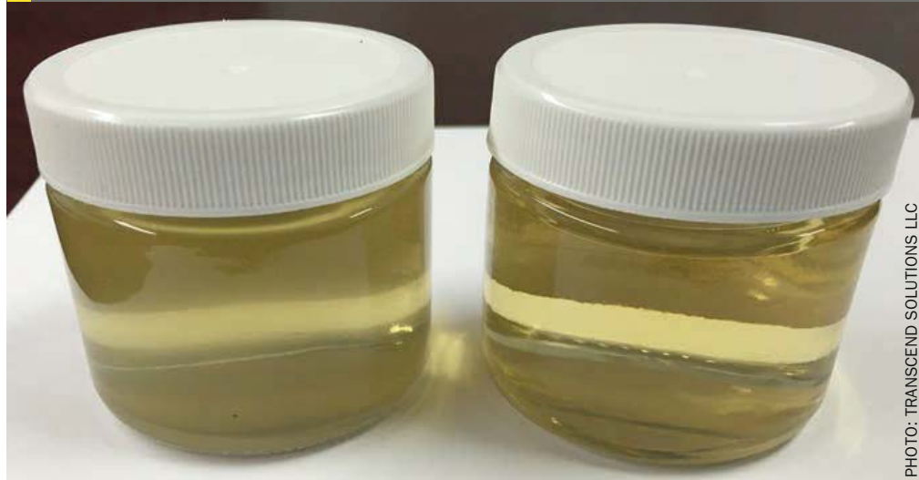
Fig. 5: (Left) Amine with emulsified hydrocarbons (Right) Amine after treatment with Envision technology
