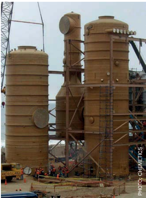
Fig. 2: Chemetics quench and scrubber venturi with variable throat design.
