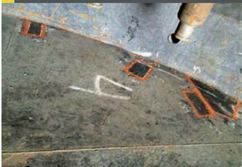
Fig. 11: Typical tank floor surface with bottom-up corrosion near perimeter
