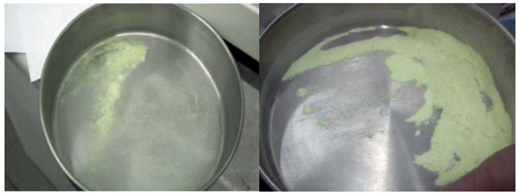
Fig. 7: Sub-300 micron sulphur retained from two samples from Ukraine.
