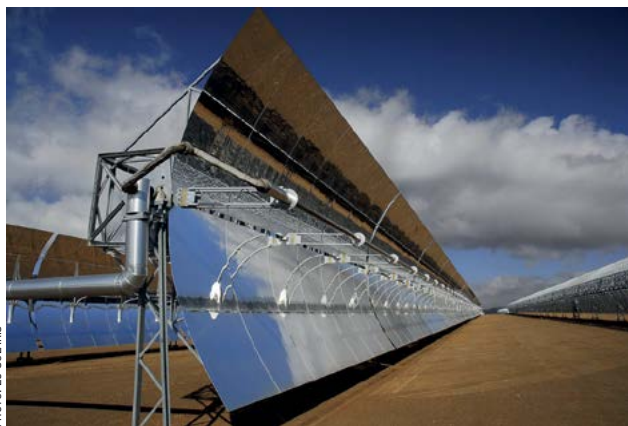
Fig. 1: Trough-shaped parabolic reflector.
