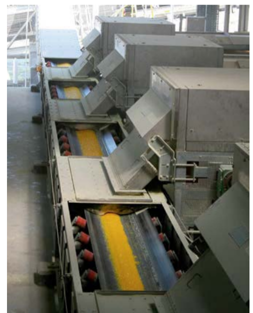
Discharge of sulphur pastilles from steel belt cooler.
