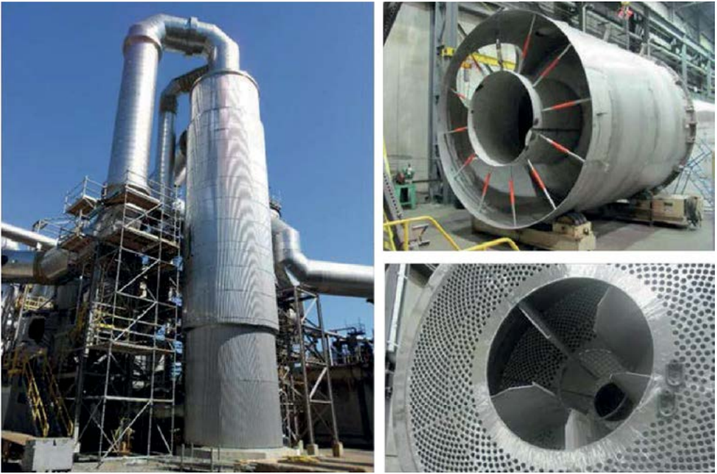
Fig. 5: Chemetics radial flow tail gas reheater installed. Unit process design developed by creating a model of current plant operation and optimizing the unit to achieve desired plant performance.
