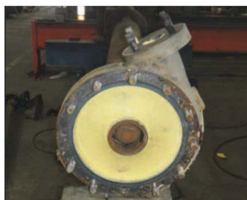
Fig. 9: Lewis® sulphur pump after removal from service, showing a heavy layer of sulphur under the suction head.
