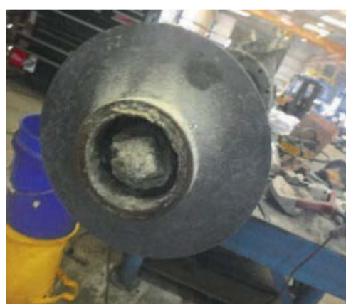
Fig. 10: Lewis® sulphur pump after cleanup – sulphur deposits still remain.
