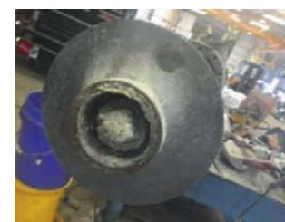
Fig. 10: Lewis® sulphur pump after cleanup – sulphur deposits still remain.
