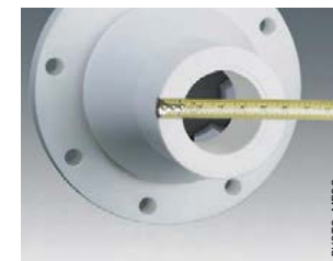
Fig. 2: A DynaWave® reverse jet nozzle after one year of continuous operation.
