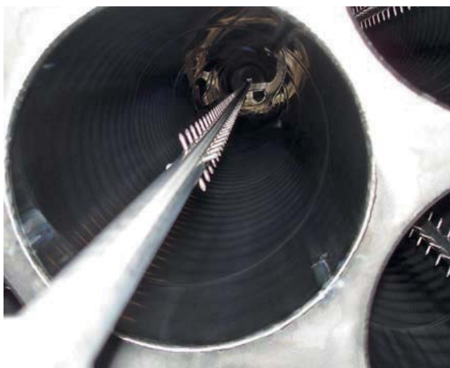
Fig. 9: Rigid mast Outotec Edirod® discharge electrode.
