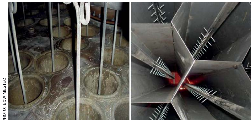
Fig. 4: Old wet ESP design using lead internals (left) versus new wet ESP design using hex tubes and rigid discharge electrodes (right).
