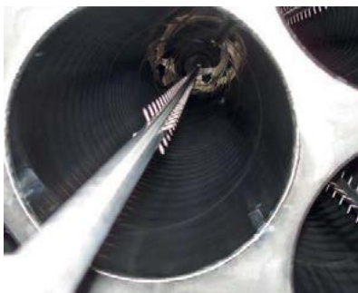
Fig. 9: Rigid mast Outotec Edirod® discharge electrode.
