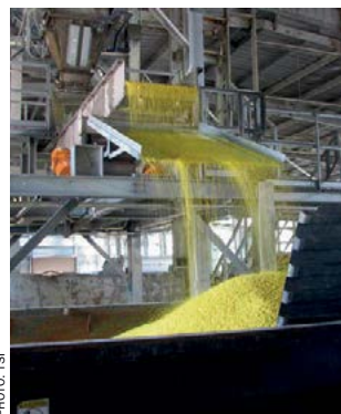
Main pic: Bulk transport of sulphur. Above: Sulphur loading into rail hopper car.
