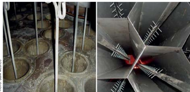
Fig. 4: Old wet ESP design using lead internals (left) versus new wet ESP design using hex tubes and rigid discharge electrodes (right).
