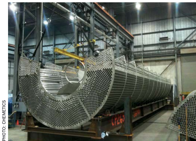
Fig. 9: Modular gas-gas heat exchanger fabrication.
