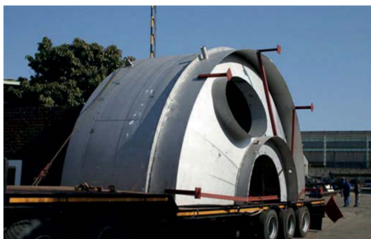
Fig. 2: Prefabricated converter modules.
