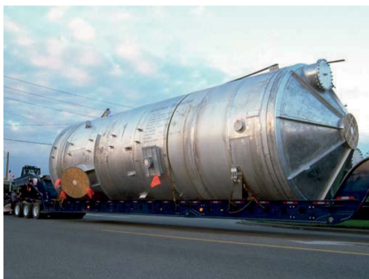
Fig. 4: Complete SARAMET® alloy acid tower.
