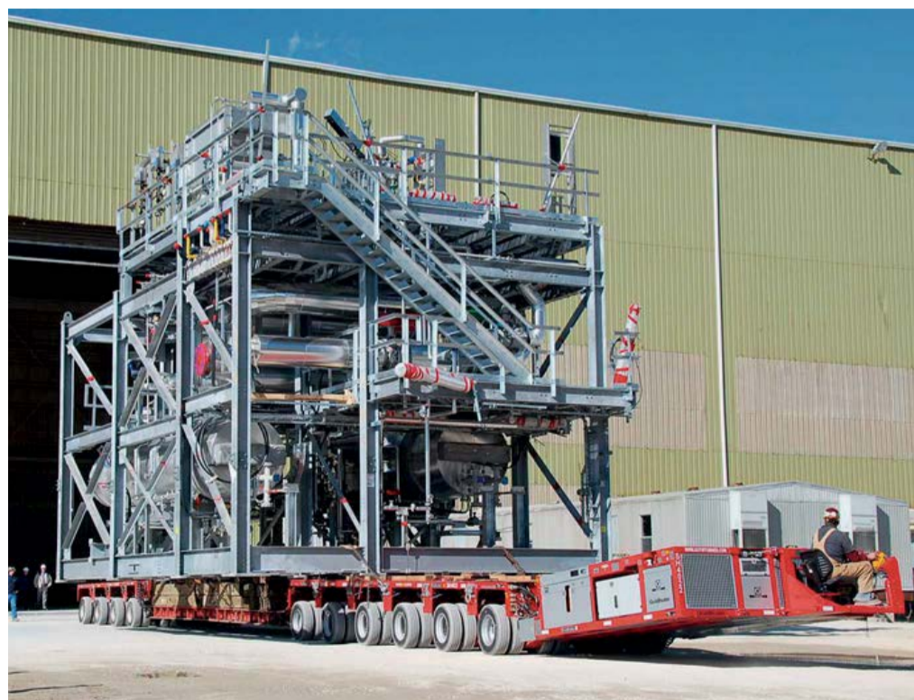
Fig. 7: Module for a 100 t/d sulphur recovery unit.
