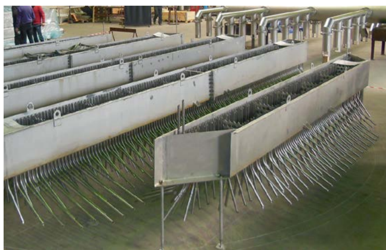
Fig. 18: NORAM trough acid distributor prior to installation.
