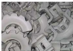
Fig. 15: Low pressure drop acid packing.
