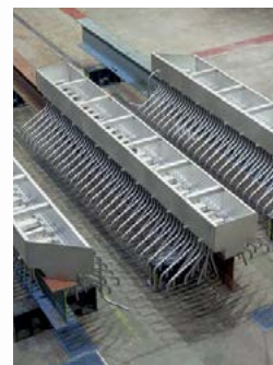
Cover: Chemetics ISO-FLOW™ Sulphuric Acid Trough Distributor with SWIFT-LOCK™. Adolfo Fernandez / Chemetics
