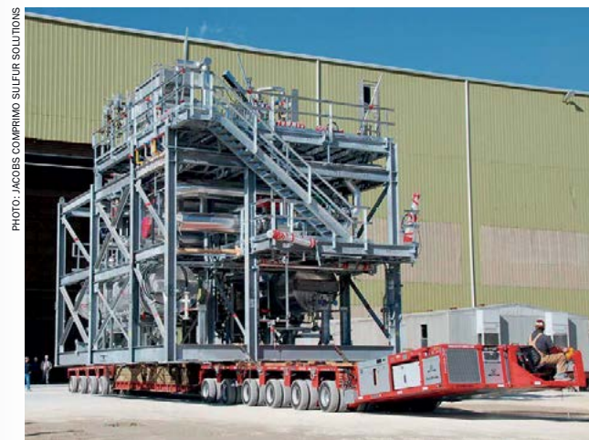
Fig. 7: Module for a 100 t/d sulphur recovery unit.
