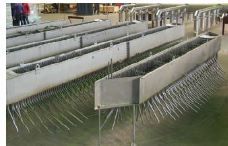
Fig. 18: NORAM trough acid distributor prior to installation.
