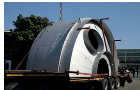
Fig. 2: Prefabricated converter modules.
