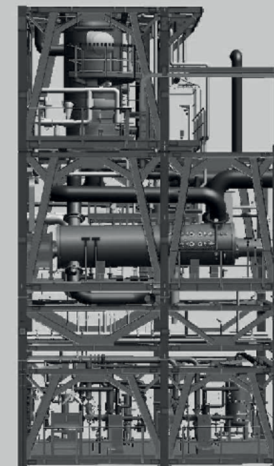
Fig. 11: TGT skid assembly containing hydrogenation reactor, inline heater, TGT waste heat boiler (on the back), filters and compact heat exchangers on the bottom.
