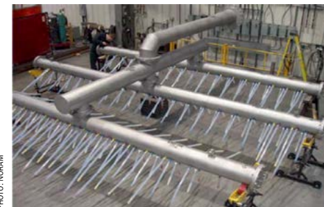
Fig. 19: Acid distributor with external clean-out nozzles.
