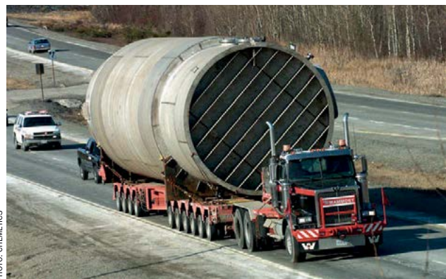
Fig. 8: Chemetics radial tube gas exchanger.
