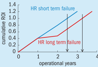
Fig 6: Cumulative ROI of a heat recovery system impacted by a failure
