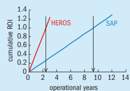
Fig 5: Cumulative ROI of a sulphuric acid plant (SAP) and a HEROS™ system
