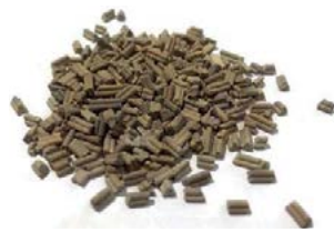
Fig. 2: S-8001 titania based low temperature TGTU catalyst is provided as extruded trilobes.
