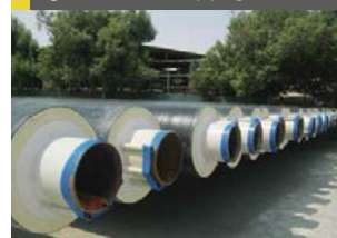
Fig 2: Pre-insulated piping sections
