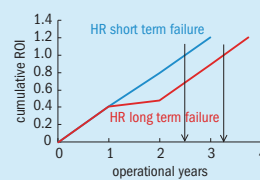
Fig 6: Cumulative ROI of a heat recovery system impacted by a failure
