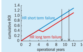
Fig 7: Cumulative ROI of a sulphuric acid plant (SAP) impacted by a HR failure
