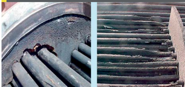
Fig 13: Reboilers corroded by excessive acid gas breakout
