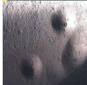
Fig 10: Hydrogen-induced cracking and blistering
