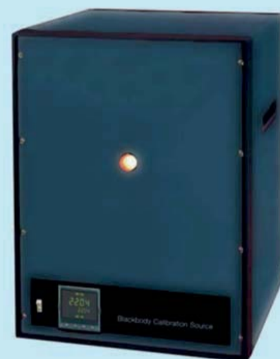
Fig 1: Commercially available blackbody calibrator
