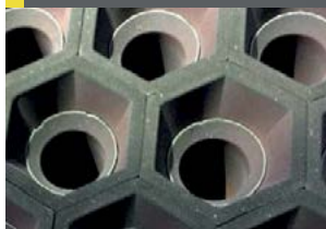
Fig 11: HexPro™ ferrules with tapered inlet for lower pressure drop
