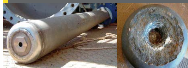
Fig 1: Sulphur gun with new spray nozzle (left) vs damaged spray nozzle (right)
