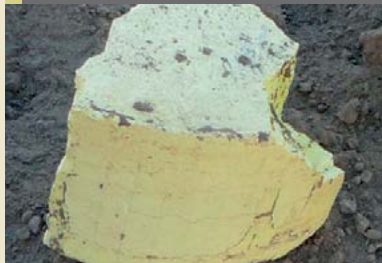
Fig 8: Hail damage – plastic covered block
