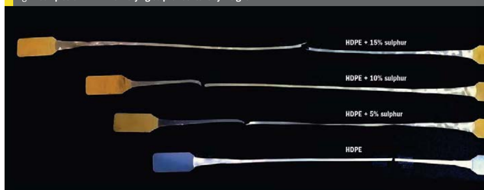
Fig 1: Samples of HDPE with varying sulphur content by weight
