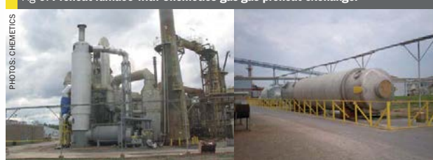
Fig 6: Preheat furnace with Chemetics gas-gas preheat exchanger
