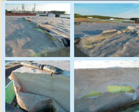
Fig 8: Hail damage – plastic covered block
