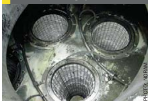
Fig 15: Hanging Brownian diffusion mist eliminator candle prewetting system
