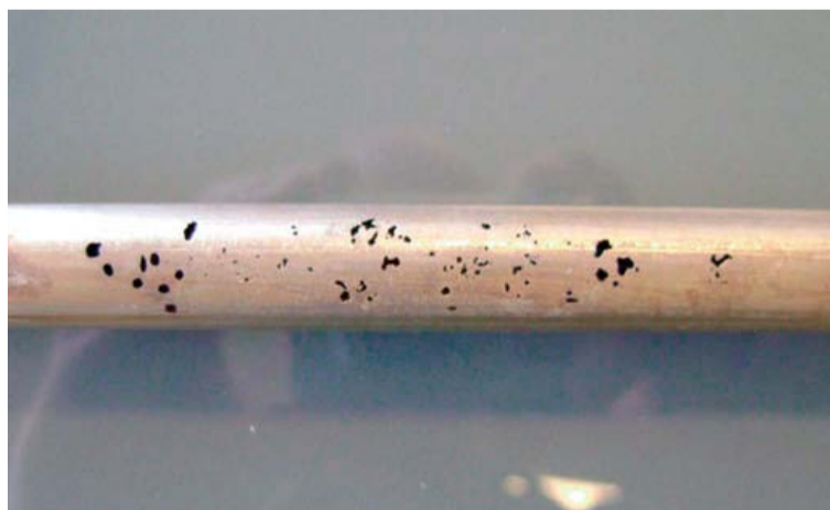
Fig. 2: Chloride water side corrosion – blocked tubing.
