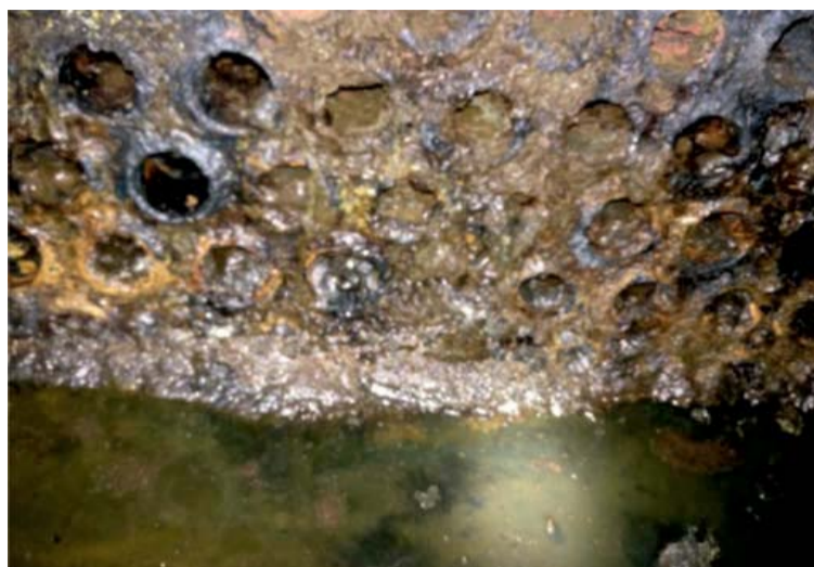
Fig. 1: Aluminised tube sheet fouled.
