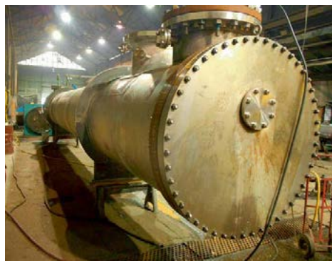
Fig. 6: Fully fabricated ZeCo ® acid cooler.
