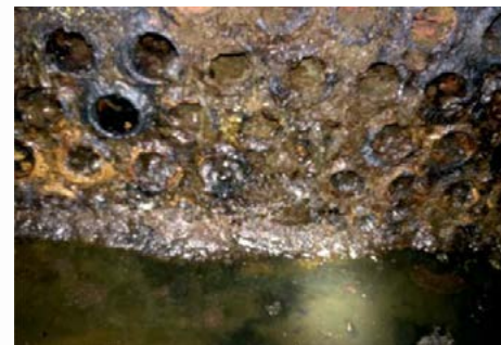
Fig. 1: Aluminised tube sheet fouled.
