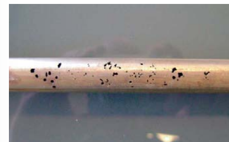
Fig. 2: Chloride water side corrosion - blocked tubing.
