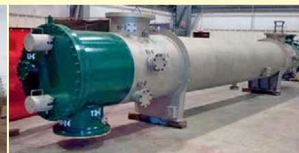
Anodically protected acid cooler.
